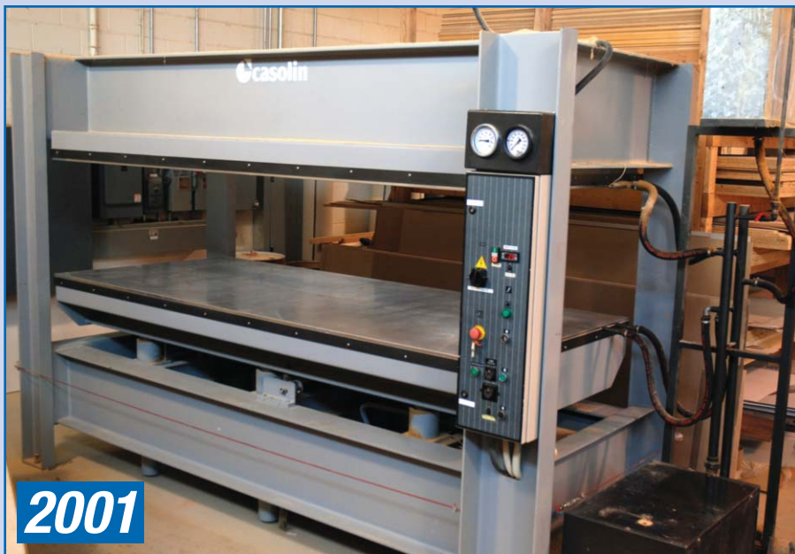
CASOLIN HEATED PLATEN PRESS, MODEL T 120
